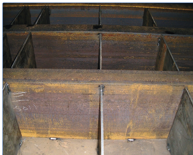
Internal construction of a large panel with deep channel section reinforcement (before welding).
